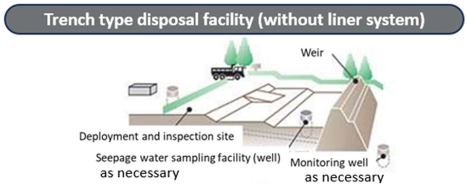
Figure XIV: Image of the final disposal facility for the removed soil and waste, which has no concern about groundwater pollution.
