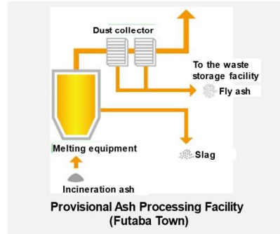
Figure VII Heat treatment methods for removed soil: burning and melting.
